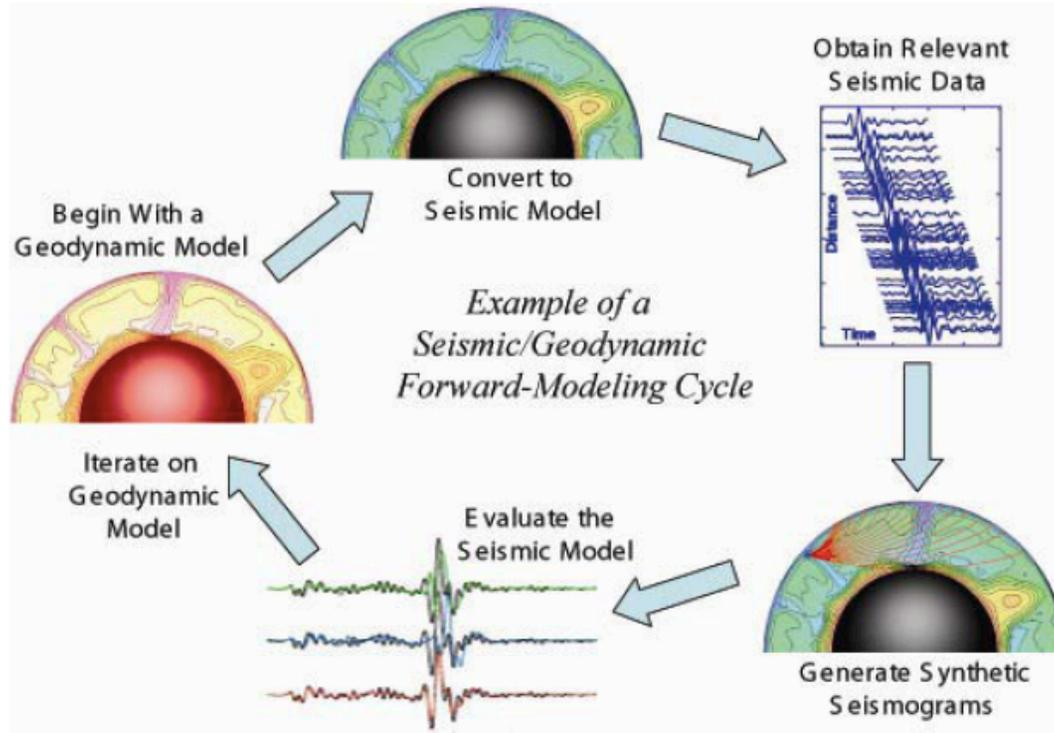
*Workflow for integrating mantle dynamics and observational seismology accomplished through a superstructure modeling framework:*
