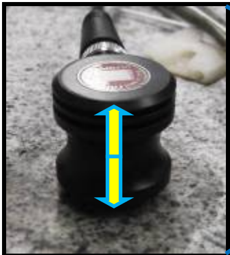
Piezoelectric sensor (detects surface normal motion)
