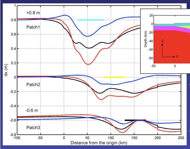
Comparison of horizontal displacements predicted from an elastic half space and from a 3D elastic model as a function the location of fault slip.
