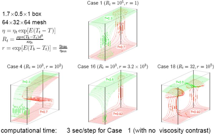
18 sec/step for Case 11 (with no Viscosity contrast) 18 sec/step for Case 18 (with 10<sup>5</sup> viscosity contrast) with Pentium IV 2.20GHz (NB: started from different initial conditions)
