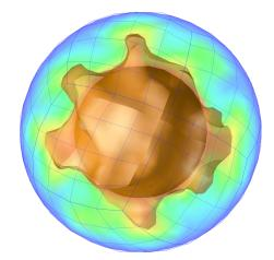
Figure 6.9: Cookbook 7: The composition and velocity field at the 15th step. The arrows are the velocity vectors. The composition field is shown in an isosurface of 0.7 and in a cross section.
