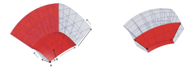
Figure 1.1: Global Node Numbering. Left: Global node numbering starts at the base of arrow A (theta\_min, fi\_min, radius\_inner), and advances from 1 at the base to *nodez* at the tip. Upon reaching the tip, numbering continues from the base of arrow B (*nodez*+1) to its tip (2 *nodez*), and so on for all nodes on the plane fi = fi\_min. Right: After completing each theta radius plane, the fi index is incremented and numbering commences from (theta\_min, radius\_inner) as on the left.
