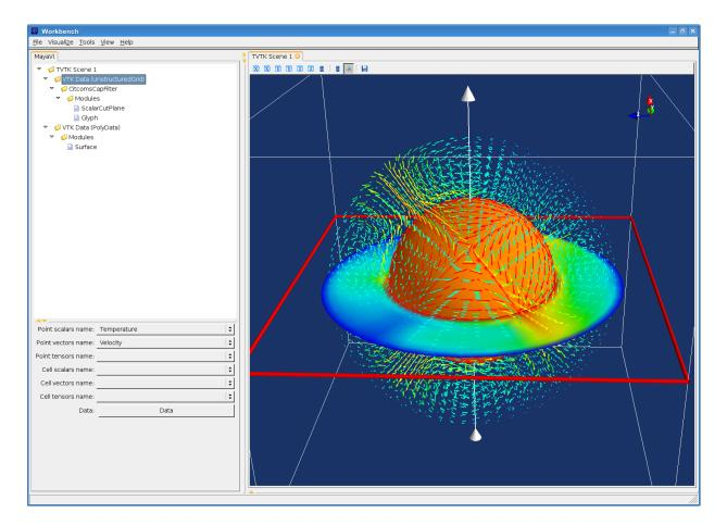
Figure 5.3: Example MayaVi2 visualization of cookbook1.100.h5. Here we display the velocity field as vectors, as well a slice of the temperature field. Note the visualization pipeline in the tree view on the left panel.
