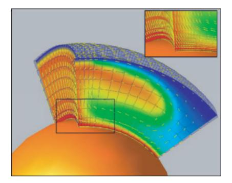
Figure 6.5: Cookbook 4: Regionally Refined Mesher. This model shows the temperature (upwelling – warm colors, downwelling – cool colors) and the uneven distribution of the velocities (yellow arrows). Note the refined mesh for the left and bottom regions of the model (inset).
