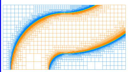
Savings from adaptive meshes are apparent. Note also the lack of numerical dispersion even without aligned meshes!
