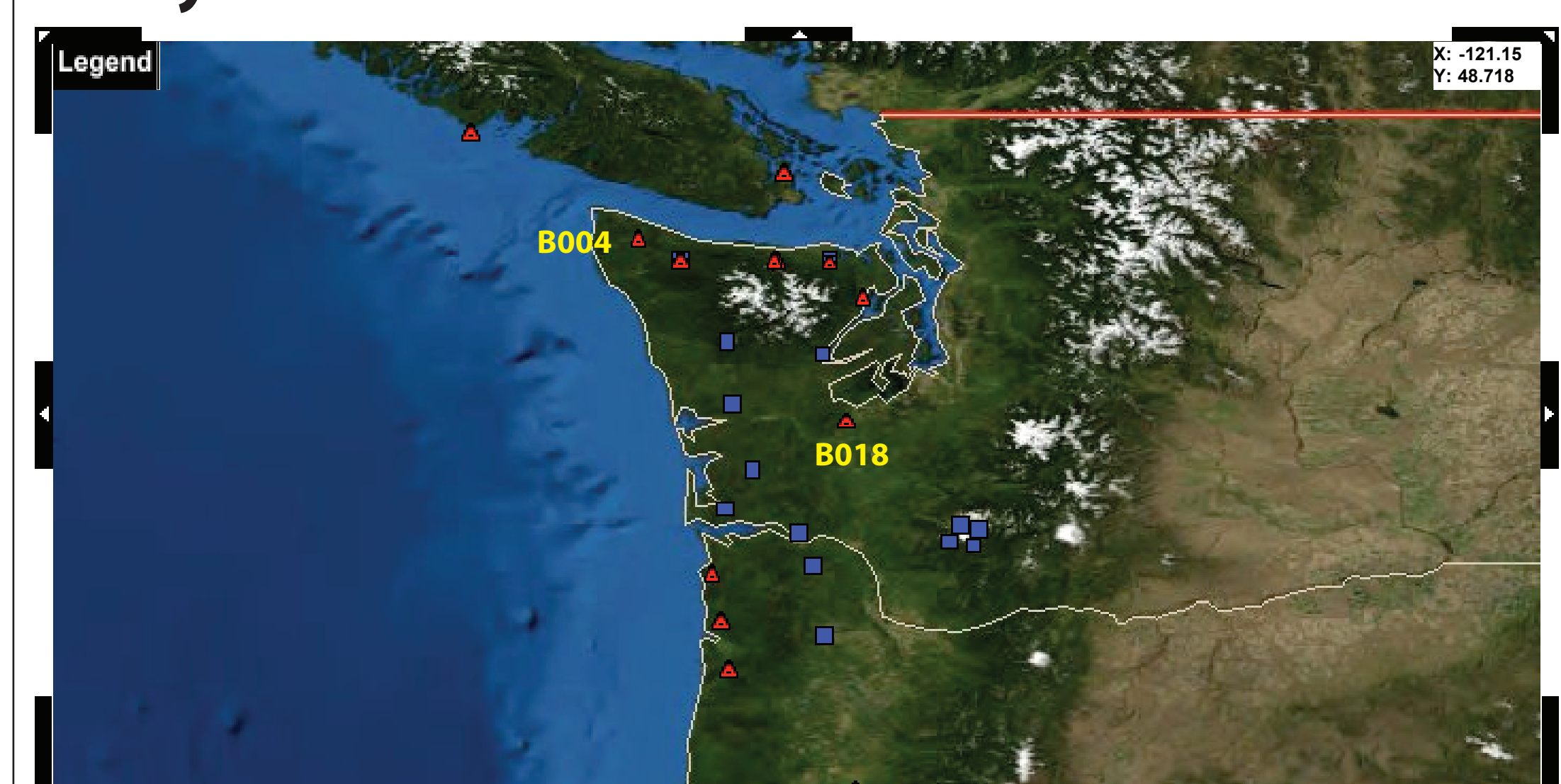
Map showing the locations of PBO borehole strainmeters in Canada, Washington, and Oregon. Red triangles show locations of currently installed and operating stations. Blue squares are planned stations. Stations B004 and B018 are labeled because they are used in the analyses at right. Map modified from Unavco/PBO website.
