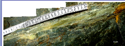
Figure 2: Rupture zone of the M2.2 earthquake, Tautona mine, South Africa. The rupture reactivated the ancient cataclastic zone of the Pretorius fault with fresh gouge (white) formation along the contact (slip localization).
